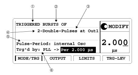
In this screen, you can set up the signal to be triggered or continuous, and to be a pulse stream or a burst (several pulses followed by a pause) consisting of single or double pulses.
