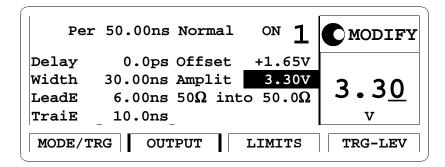
Here is the figure as displayed on the Agilent 54810A Infinium oscilloscope. Use the generator's TRIGGER OUT to trigger the scope.
