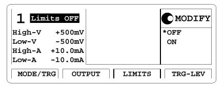
After you switch on the limits, the pulse level parameters on the OUTPUT screen cannot be adjusted outside the ranges specified on the LIMITS screen if the output is switched on. Note that because current and voltage limits apply, the available ranges of the impedance parameters are also affected.
