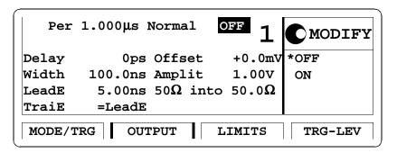
Press the OUTPUT softkey to access this screen.
