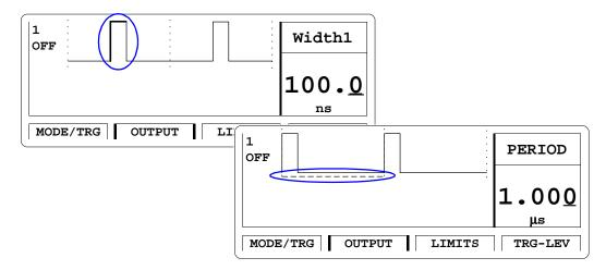
Use the left/right cursor keys to toggle between the individual timing parameters.
