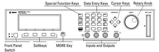
The **front panel switch** is used to switch on and off the instrument.
