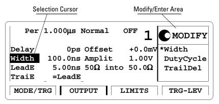
The available formats for the pulse width parameter are displayed in the Modify/Enter area.
