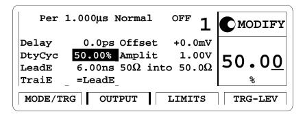
If you need to specify a unit for a parameter, simply press the appropriate unit key (NANO, MICRO/MEGA, MILLI/KILO) instead of the ENTER key.
