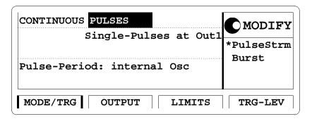
Press the MODE/ TRG softkey to access this screen. In this screen, you can set up the signal to be triggered or continuous, and to be a pulse stream or a burst (several pulses followed by a pause) consisting of single or double pulses.
